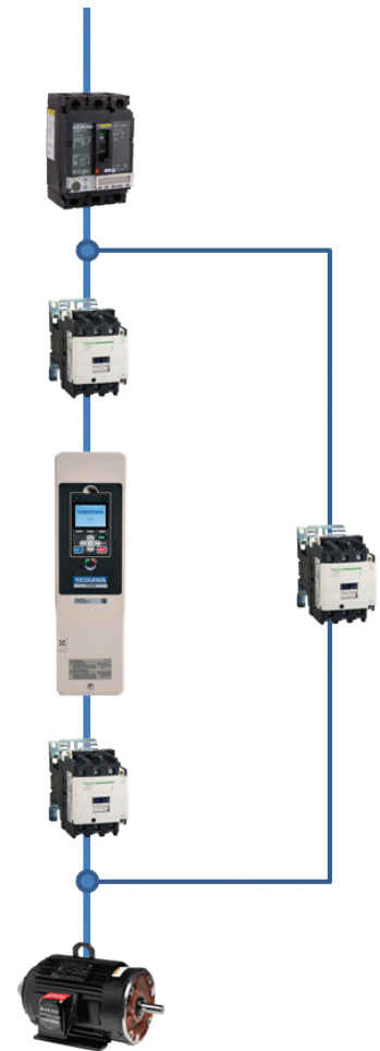
Figure 13: Three-contactor bypass setup
