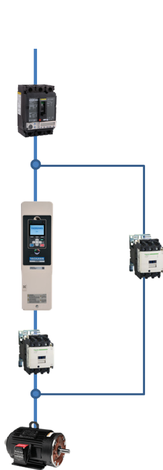
Figure 12: Two-contactor bypass setup
